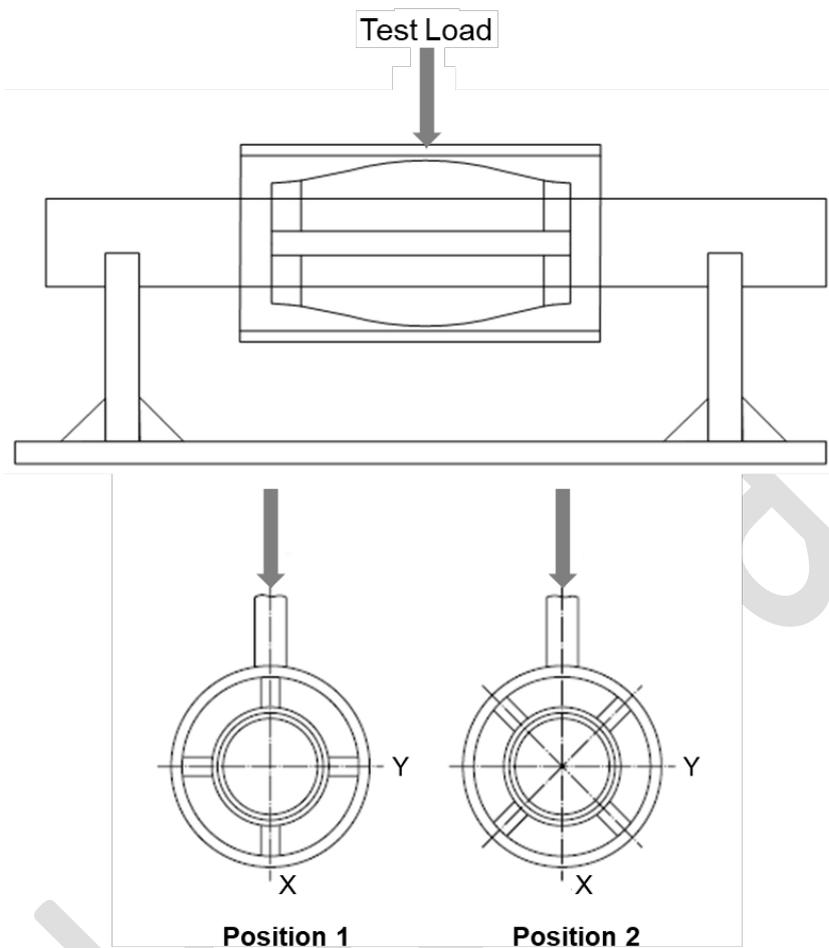
**Figure 6—Standoff Test & Bow-Spring Casing Centralizer Test positions**
