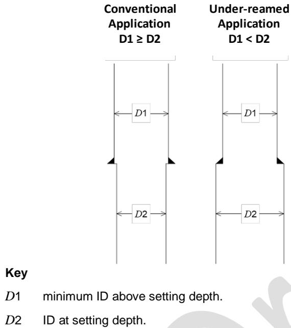
Figure 1—Conventional and Under-reamed Bow-spring Centralizer Applications
